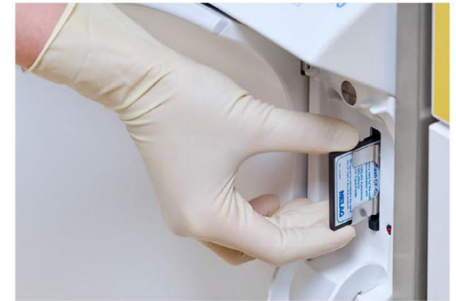
MELAG washer-disinfectors monitor all the relevant process parameters to ensure the highest-possible level of safety. The generated logs **provide legal certainty and can be saved via CF card or two network interfaces.**
