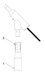
The stand post comes with a fully retracted telescoping tube. As the telescope has an integrated spring counterbalance system that keeps the mounted light body exactly in the desired location, for transport reasons, it is secured by screw 1 in its fully retracted position. This screw is to be removed in the following manner: Hold the telescoping tube steady and after removing the screw, allow it to slowly extend until it is all the way out.
