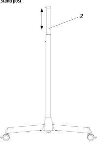
The height of the stand post can be infinitely adjusted with just one hand and remains precisely positioned at the desired height.
