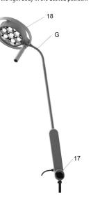
**Caution!** Positioning the KaWe examination light at an angle of less than 90° is not allowed as this may damage the flexible hose connection.
