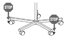
• To move the light, release the brakes on the castors
